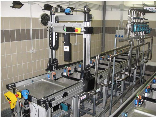
**Figure 3.12:** One of the six automated chains of the film development facility at the external LNGS laboratory
