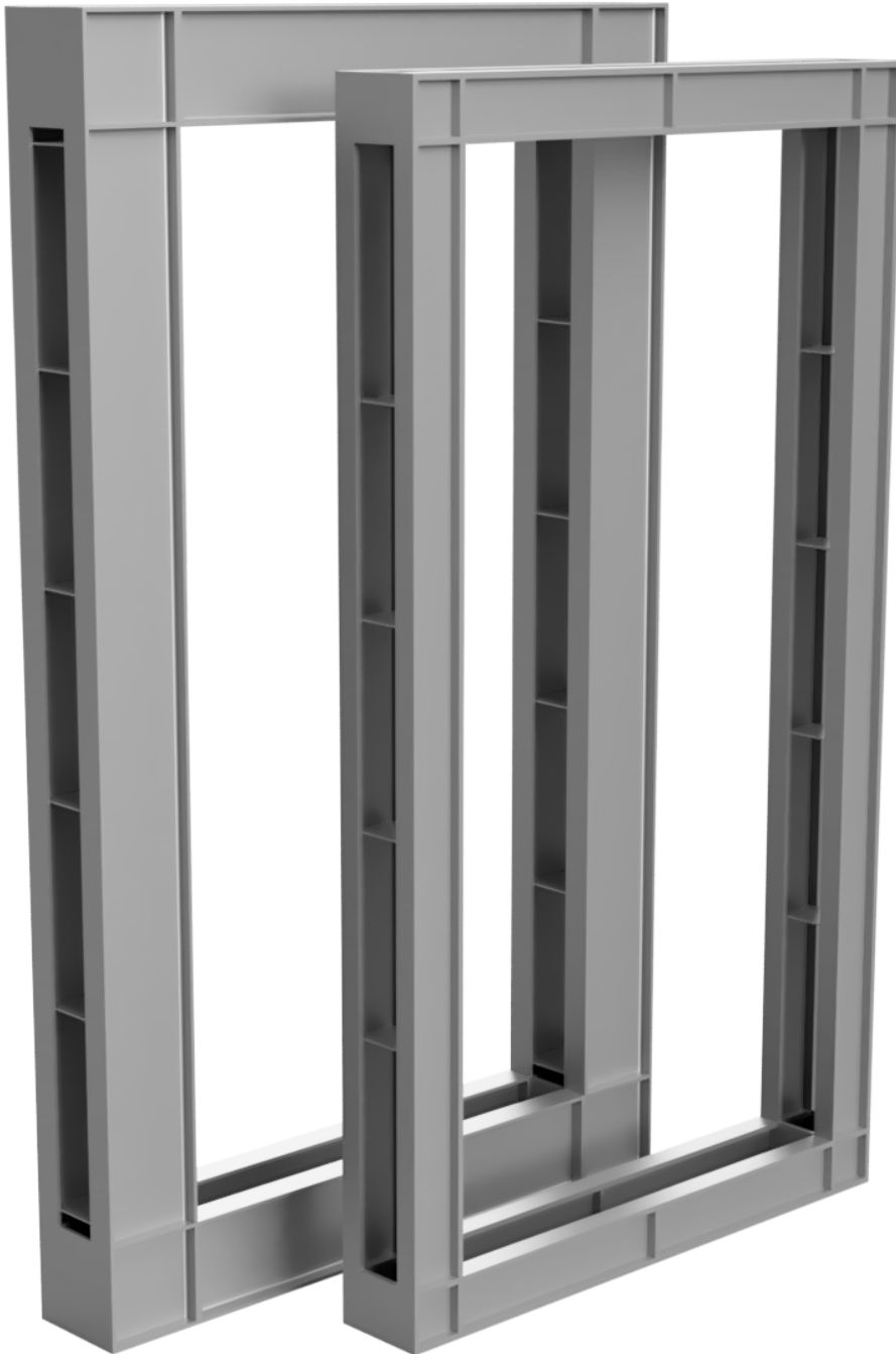
Figure 8.13: Comparison between the larger and the smaller frame. The smaller frame is 0.54 m less tall, 0.696 m less wide and 0.114 m less deep. Otherwise, the basic design features such as the intermediate floors are similar.
