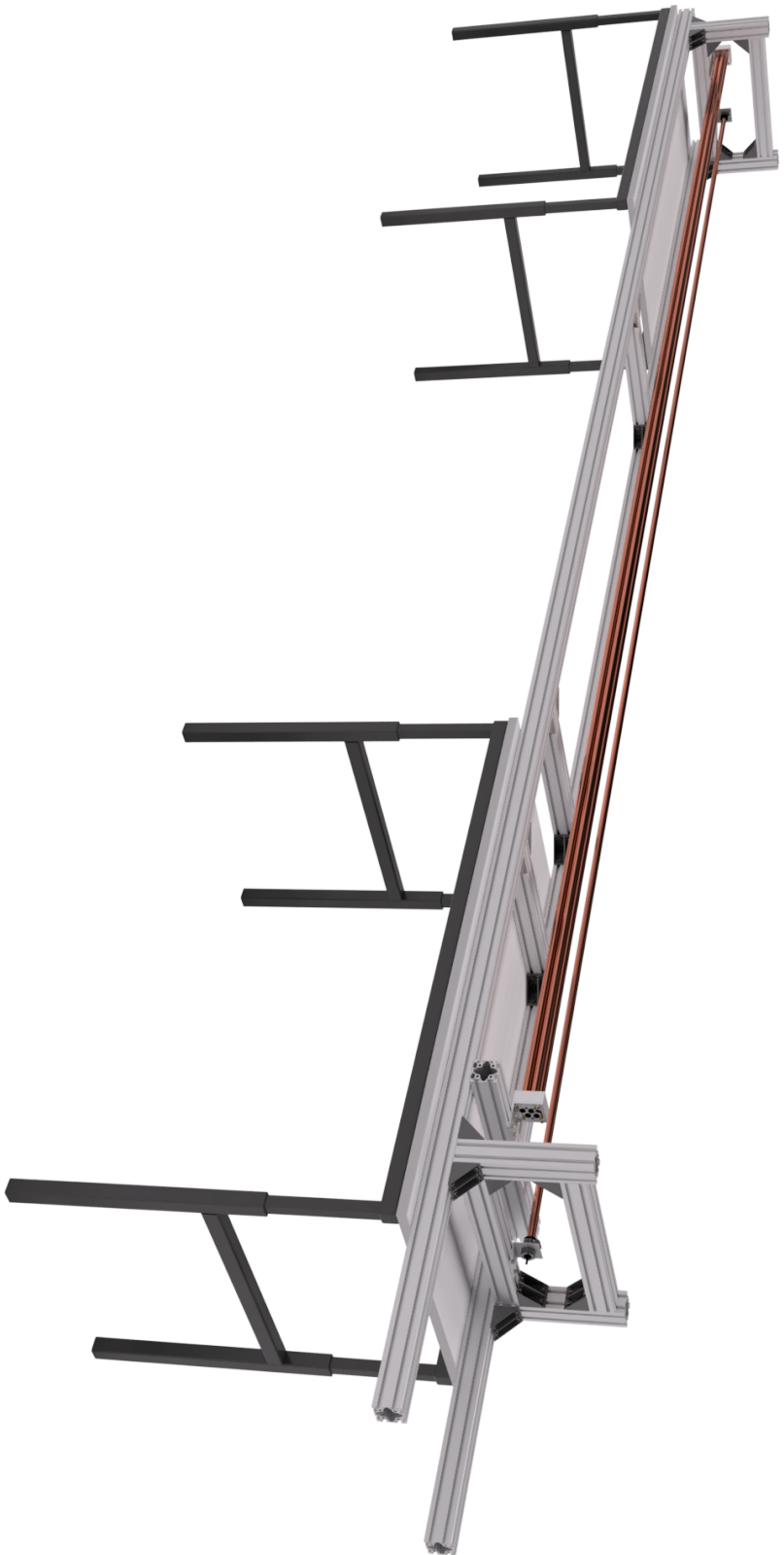
Figure 6.11: The assembled quad-straw prototype next to the single-straw functional model on the mounting frame. For the quad-straw prototype the ends of the straw tubes were cut off, resulting in the quad-straw prototype being slightly shorter than the single-straw functional model. Thus, one end of the quad-straw prototype is mounted to an additional, offset aluminium profile. The carbon fibre tows as well as the carbon spacers were not yet installed. The electronics and gas system are not depicted in this image.
