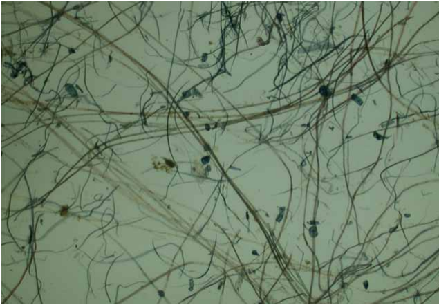
Fig. 5: Paper of the Cone Kanjur in volume 1 mdo shows the presence of paper mulberry and straw fibres in 60x magnification.
