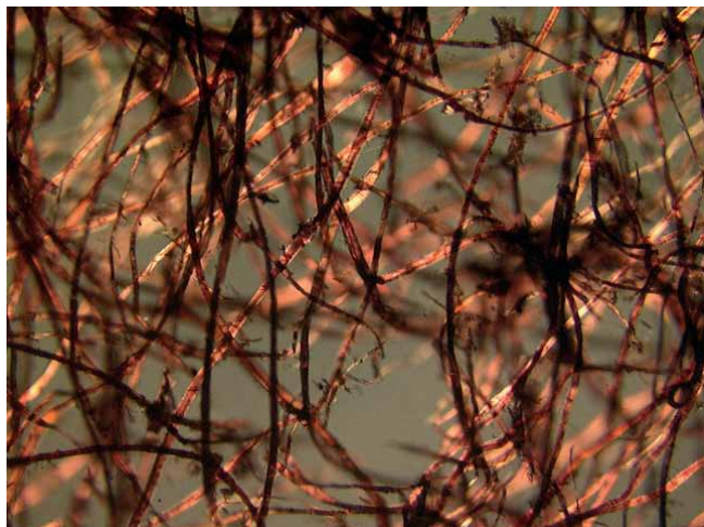
Fig. 3: Paper mulberry fibres in polarized light visible on image at 150 x magnification composing the paper of the Wanli Kanjur (vol. 60 of the Pander Pantheon collection) from the Jagiellonian University Library, Cracow.
