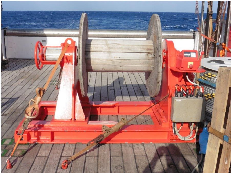
Picture: Portable storage winch with wooden empty drum
