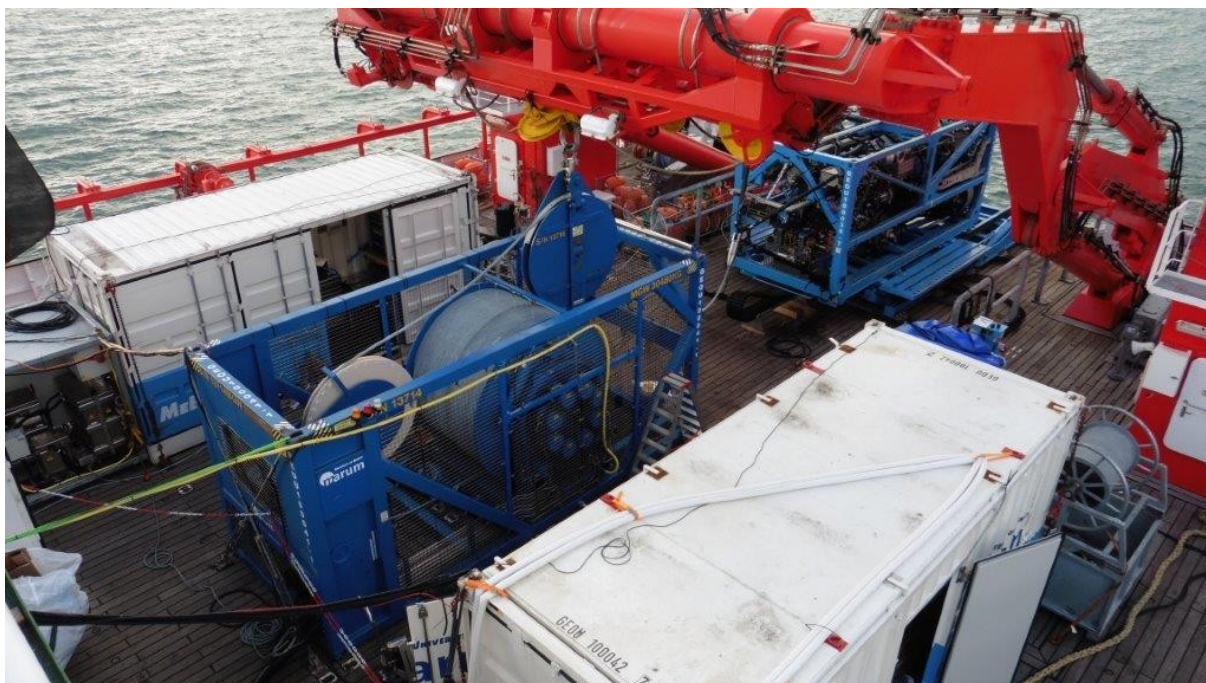
Arrangement MeBo 200 in the area of the A-Frame
