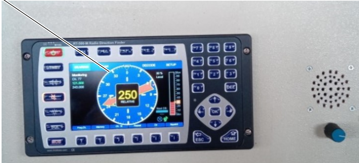
Fig. 113 RhoTheta 500 radio direction finder, Gonio radio direction finder
